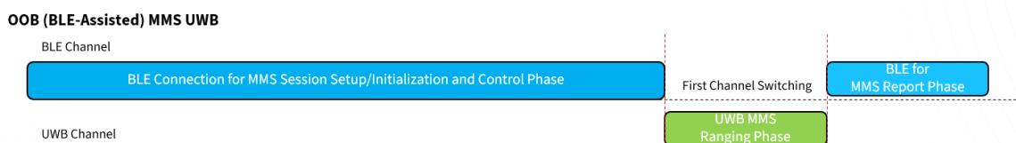
Figure 23: OOB (BLE-Assisted) MMS UWB
